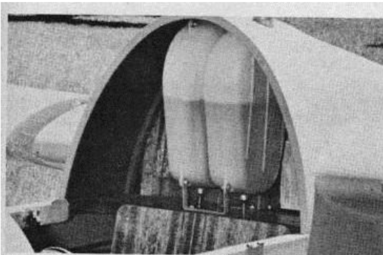
The fuel tanks located behind the pilot are plastic.
