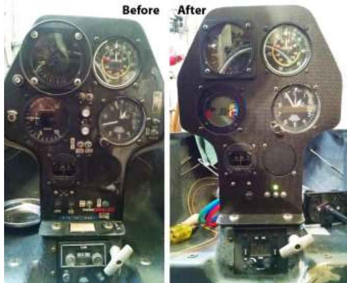
**Synopsis:** Making your existing fiberglass or aluminum instrument panel into a carbon fiber look and feel panel is easy – and it looks sharp too! John DeRosa will show the two ways that this can be accomplished with the tools and procedures needed.
